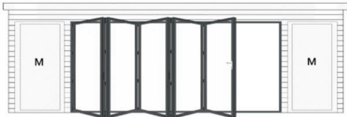
24' (7.12m) front with 14ft 5-leaf bifold door & 2 (M) 850mm fixed windows to front
