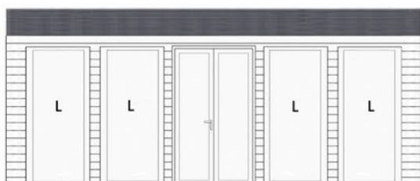
22' (6.71m) front with 1285mm double doors with 4 (L) 1000mm fixed windows
