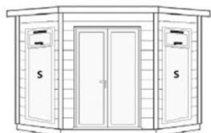
6' (1.83m) front with French full length double doors & 2 (S) 515mm opening windows to front
