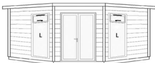
13' (3.96m) front with French full length double doors & 2 (L) 1180mm opening windows to front
