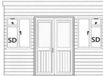
12' (3.66m) front with 1285mm double doors with 2 (SD) 915mm opening windows
