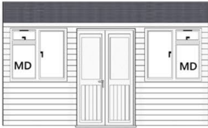
16' (4.88m) front with 1285mm double doors with 2 (MD) 1200mm opening windows
