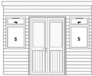
10' (3.05m) front with 1285mm double doors with 2 (S) 600mm opening windows
