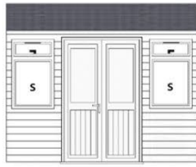
10' (3.05m) front with 1285mm double doors with 2 (S) 600mm opening windows
