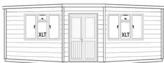
13' (3.96m) front with French 1/2 length double doors & 2 (XLT) 1800mm opening windows to front
