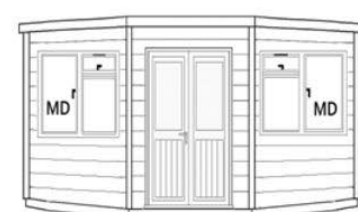
9' (2.74m) front with French 1/2 length double doors & 2 (MD) 1400mm opening windows to front
