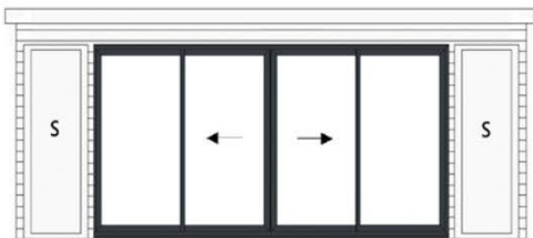
22' (6.71m) front with 14ft double sliding door & 2 (S) 600mm fixed windows to front
