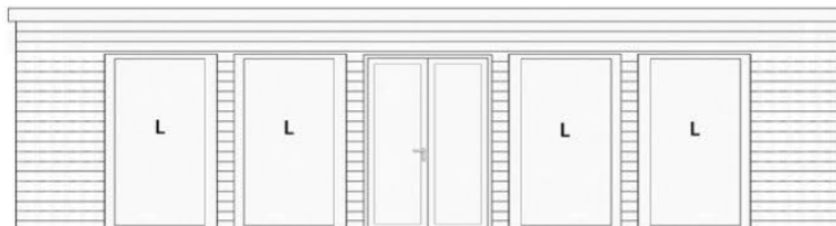
30' (9.14m) front with 1285mm double doors with 4 (L) 1400mm fixed windows
