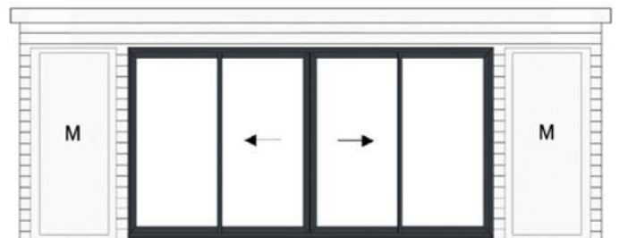
24' (7.12m) front with 14ft double sliding door & 2 (M) 850mm fixed windows to front
