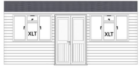
20' (6.10m) front with 1285mm double doors with 2 (XLT) 1800mm opening windows
