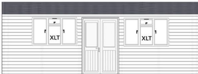
26' (7.92m) front with 1285mm double doors with 2 (XLT) 1800mm opening windows
