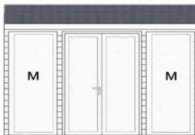
12' (3.66m) front with 1285mm double doors with 2 (M) 900mm fixed windows
