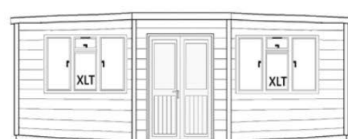
12' (3.66m) front with French 1/2 length double doors & 2 (XLT) 1800mm opening windows to front
