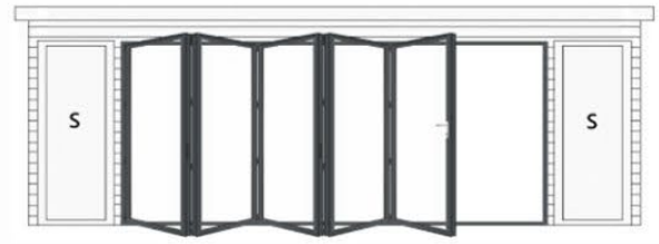
22' (6.71m) front with 14ft 5-leaf bifold door & 2 (S) 600mm fixed windows to front
