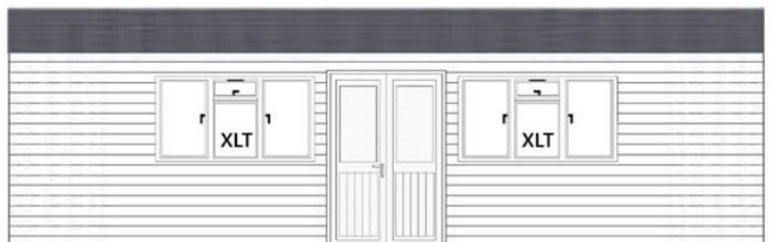
30' (9.14m) front with 1285mm double doors with 2 (XLT) 1800mm opening windows
