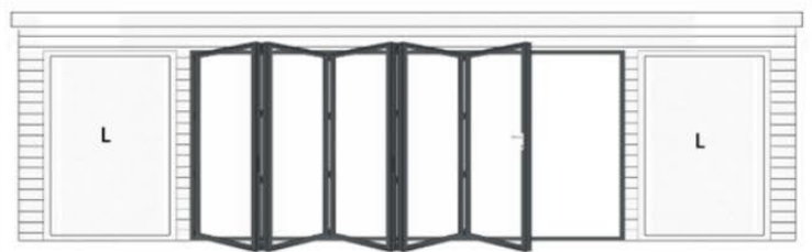
26' (7.92m) front with 14ft 5-leaf bifold door & 2 (L) 1100mm fixed windows to front
