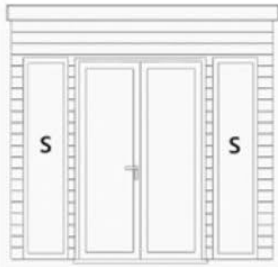
8' (2.44m) front with 1285mm double doors with 2 (S) 320mm fixed windows
