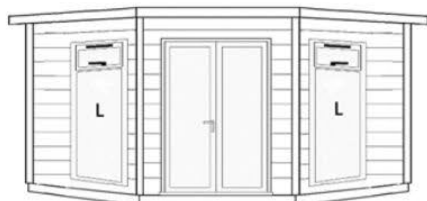
10' (3.05m) front with French full length double doors & 2 (L) 1180mm opening windows to front
