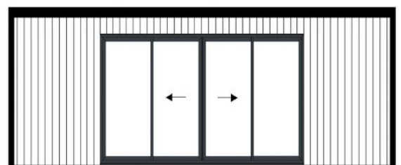
22' (6.71m) front with 12ft double sliding door
