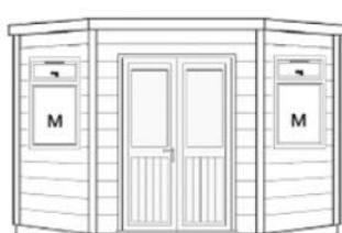
7' (2.13m) front with French 1/2 length double doors & 2 (M) 800mm opening windows to front
