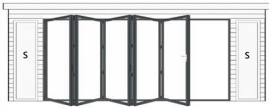
20' (6.10m) front with 14ft 5-leaf bifold door & 2 (S) 400mm fixed windows to front
