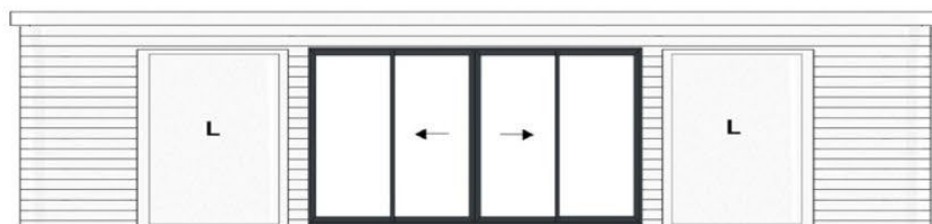
30' (9.14m) front with 14ft double sliding door & 2 (L) 1400mm fixed windows to front
