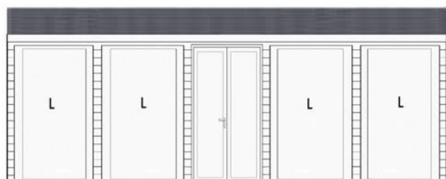
24' (7.12m) front with 1285mm double doors with 4 (L) 1200mm fixed windows
