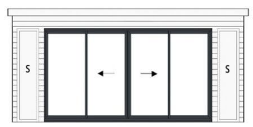
20' (6.10m) front with 14ft double sliding door & 2 (S) 400mm fixed windows to front
