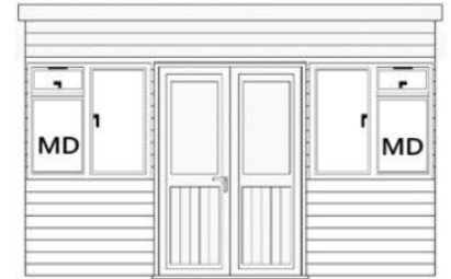
14' (4.27m) front with 1285mm double doors with 2 (MD) 1200mm opening windows
