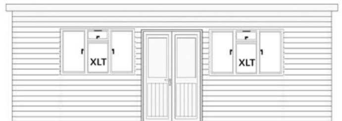
24' (7.12m) front with 1285mm double doors with 2 (XLT) 1800mm opening windows
