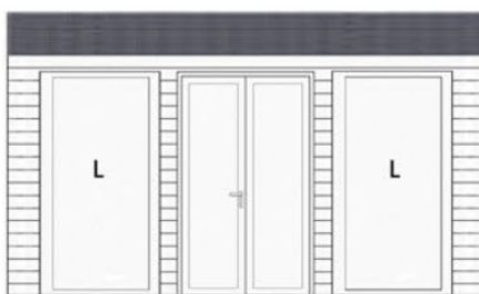
18' (5.49m) front with 1285mm double doors with 2 (L) 1400mm fixed windows
