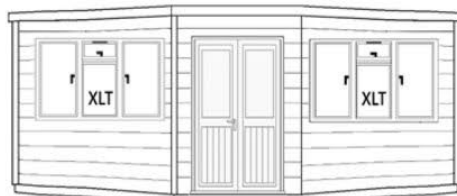
11' (3.35m) front with French 1/2 length double doors & 2 (XLT) 1800mm opening windows to front
