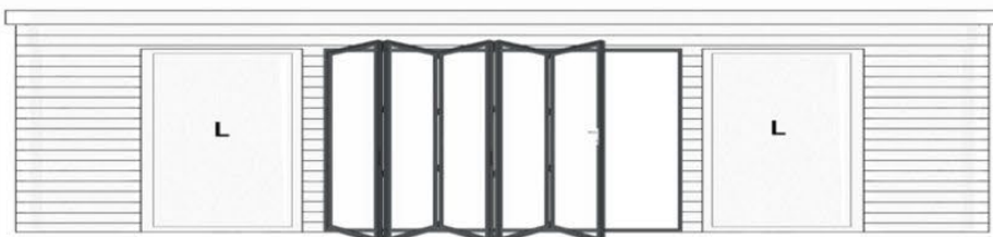
30' (9.14m) front with 14ft 5-leaf bifold door & 2 (L) 1400mm fixed windows to front
