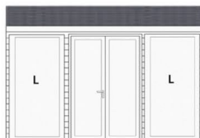
14' (4.27m) front with 1285mm double doors with 2 (L) 1200mm fixed windows
