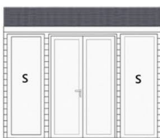
10' (3.05m) front with 1285mm double doors with 2 (S) 600mm fixed windows
