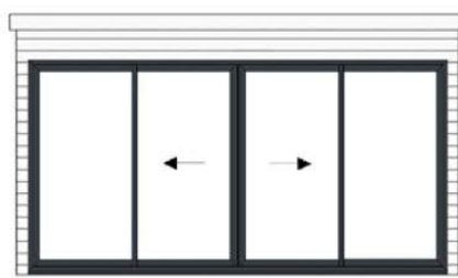
18' (5.49m) front with 14ft double sliding door
