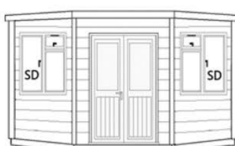
8' (2.44m) front with French 1/2 length double doors & 2 (SD) 1100mm opening windows to front
