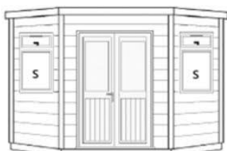
6' (1.83m) front with French 1/2 length double doors & 2 (S) 515mm opening windows to front
