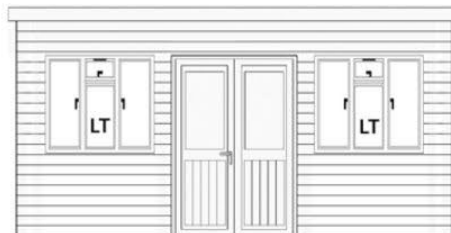
18' (5.49m) front with 1285mm double doors with 2 (LT) 1600mm opening windows
