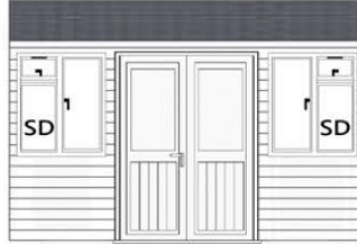
12' (3.66m) front with 1285mm double doors with 2 (SD) 915mm opening windows
