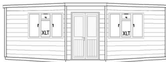
14' (4.27m) front with French 1/2 length double doors & 2 (XLT) 1800mm opening windows to front
