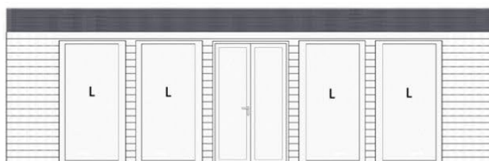
30' (9.14m) front with 1285mm double doors with 4 (L) 1400mm fixed windows
