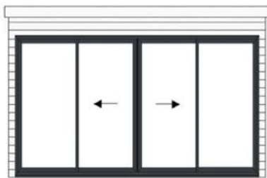
16' (4.88m) front with 14ft double sliding door
