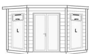
8' (2.44m) front with French full length double doors & 2 (L) 1100mm opening windows to front
