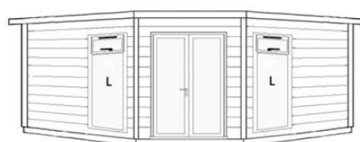
14' (4.27m) front with French full length double doors & 2 (L) 1180mm opening windows to front
