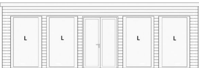
26' (7.92m) front with 1285mm double doors with 4 (L) 1400mm fixed windows
