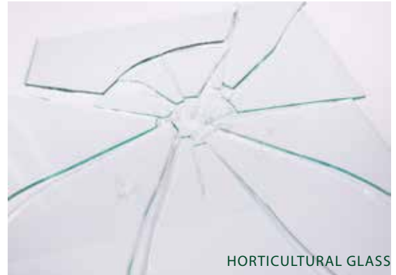
HORTICULTURAL GLASS Breaks into large shards which can be dangerous.
