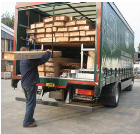
Height: 11'4", Length: 30', Width: 8'6" Class II - 15 tonne (similar in dimension to a furniture removal van)
