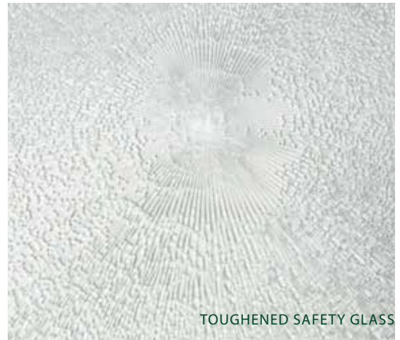
TOUGHENED SAFETY GLASS Breaks into small granules which is less likely to cause injury.
