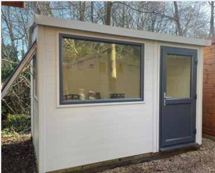
10' X 8' Apex garden studio. thermowood cladding, UPVC doors & windows slate grey, satin handles & levers & grey hinges, half length single door, half length opening window (1000 x 1200) & half length fixed window (1000 x 1400), double glazed, MDF (V grooved) painted lining (white) with breathable membrane (moisture barrier) & Celotex insulation, painted finish in elephant grey, EPDM rubber roof, laminate floor midnight grey.
