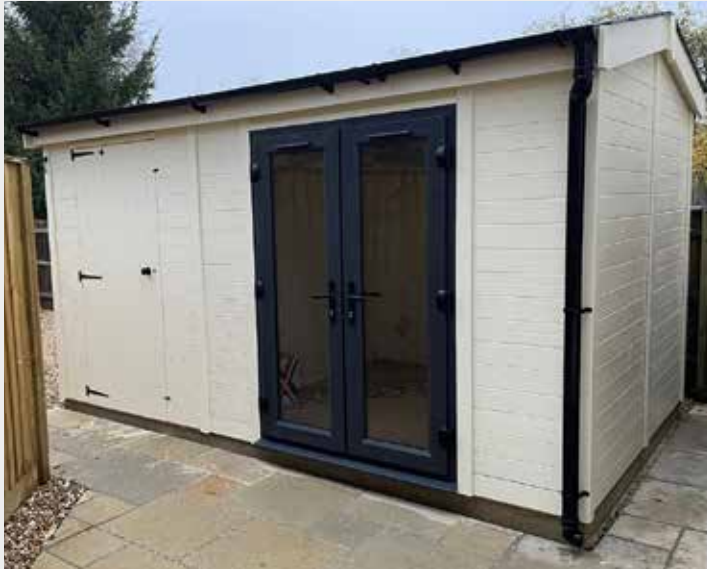
13' x 8' Apex garden studio. Thermowood cladding, UPVC doors & windows in anthracite grey, full length glazing, double glazed glass, MDF (V grooved) painted lining (White) with breathable membrane (moisture barrier) and Celotex insulation, painted finish in Linen, slate effect tile roof, laminate floor, black guttering, black handles & levers.
