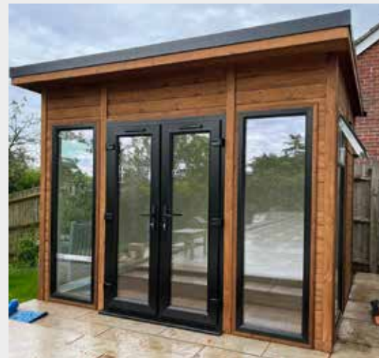
10' X 8' Pent garden studio, thermowood cladding, UPVC doors & windows black external, white internal, full length double doors with 2 fixed full length windows (710 x 1857) & 2 opening top lite full length windows (710 x 1857), door hinges, handle & window levers black, MDF (V grooved) painted lining (white), with breathable membrane (moisture barrier) and Celotex insulation, solvent treated, EPDM rubber roof, laminate floor in farmhouse summer oak & black guttering
